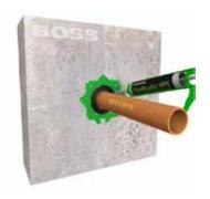
4. Tool the sealant with a wet pallet knife or trowel, flush with the wall surface. Then remove the masking tape.
