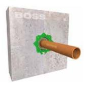
Apply the sealant around the service and fill the void to the surface of the wall. Best results are achieved if filling the void is started at the bottom of the void and work upwards.
