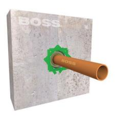
3. Apply the sealant around the service and fill the void to the surface of the wall. Best results are achieved if filling the void is started at the bottom of the void and work upwards.
